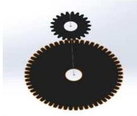
Figure 1: Part assembly of the spur gear prepared in solid works
